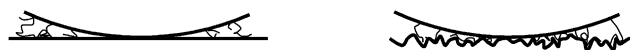
Fig. 6. A schematic depiction of the interactions between rough and smooth substrates. When an easily deformable layer covers the particle, the effective contact surface area is increased, not decreased, as is the case with a hard, rigid particle.
